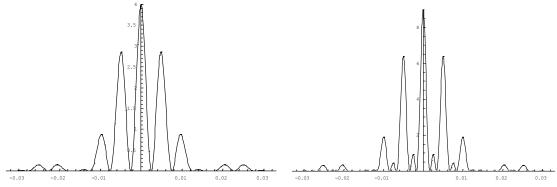
Above are plots of the diffraction pattern for a (left) 2-slit (b=0.04 mm, a=.125 mm) and (right) 3-slit (b=0.04 mm, a=.125 mm) illuminated with He-Ne laser light at 632.8 nm.
